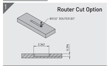
Use a Ø9/32" router bit to cut a slot in both substrates where the Hook and Key of the Mini 60 is to be mounted. Depth needs to be 0.394" for each.
