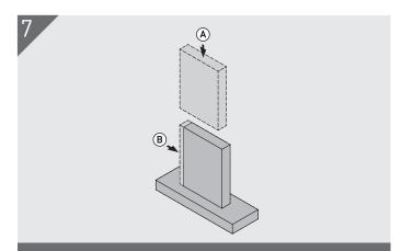
Assembly components remembering the Key only needs to travel 1 pitch for full engagement. This is detailed in steps A and B.
